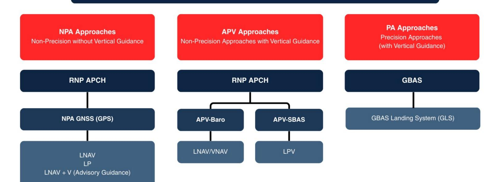
LNAV+V provides advisory vertical guidance only. It creates an artificial glide path to help maintain a constant descent to MDA but is not the same as LNAV/VNAV or LPV.
